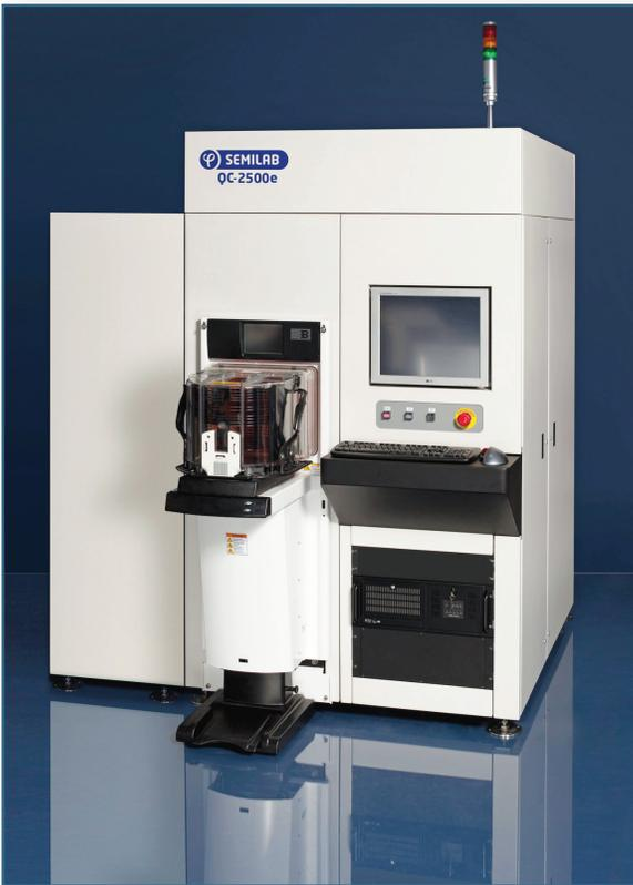
The QC-2500e near surface doping mapper from Semilab uses non-contact technology to measure near-surface resistivity, doping concentration and recombination lifetime on epitaxial wafers. The fully automated platform features a LowBoy linear positioning stage to quickly and precisely move wafers into position for inspection by optical lasers.
