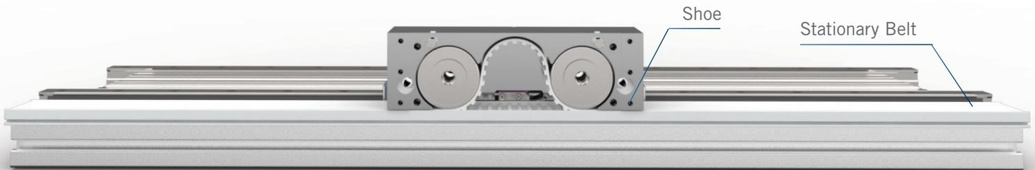
ServoBelt™ Linear comes in two different carriage styles. The *Standard* carriage is more compact and uses our dual-belt drive technology. This carriage style is suitable for most applications. The *LoopTrack* carriage is a design in which the upper drive belt loops continuously within the carriage itself. It prevents the possibility of belt sag in inverted or cantilevered applications.
