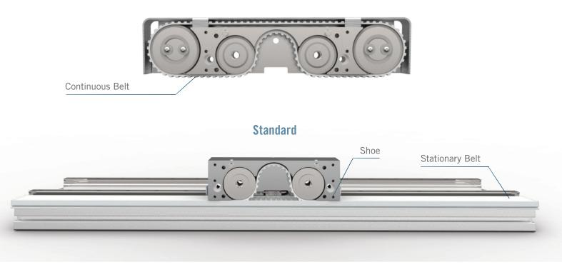
ServoBelt<sup>™</sup> Linear comes in two different carriage styles. The *Standard* carriage is more compact and uses our dual-belt drive technology. This carriage style is suitable for most applications. The *LoopTrack* carriage is a design in which the upper drive belt loops continuously within the carriage itself. It prevents the possibility of belt sag in inverted or cantilevered applications.
