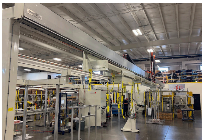
The ServoBelt-powered gantry spans multiple machining centers, transporting camshafts through sequential operations.
