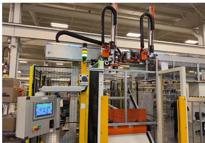
The complete gantry system includes ServoBelt technology, a composite beam and custom safety features to deliver automotive-grade performance.
