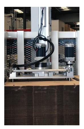
The safety guarding, which is based on a simple arrangement of overhead sliding gates and sensors that lock out the robot from the machine below, cost just a fraction of what a floor-mounted 6-axis robot would require.
