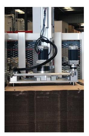
The safety guarding, which is based on a simple arrangement of overhead sliding gates and sensors that lock out the robot from the machine below, cost just a fraction of what a floor-mounted 6-axis robot would require.
